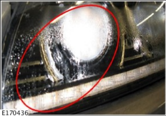
In the photograph shown below, note the standing water within the lamp
