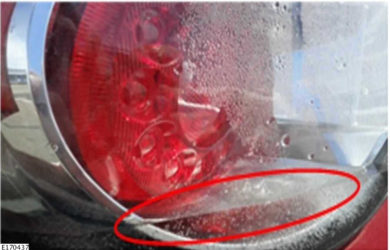
In the photograph shown below, note the thick mist covering the lens with water droplets
